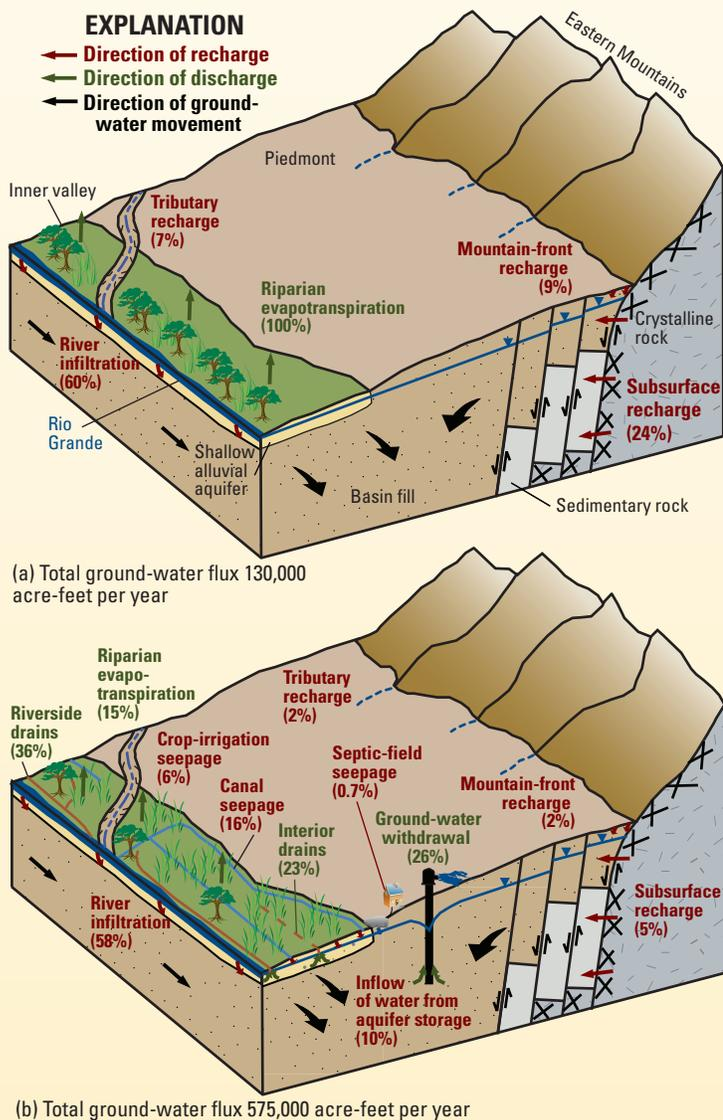
**Figure 2.** Generalized block diagram for the Middle Rio Grande Basin, New Mexico, showing components of the ground-water system under (a) predevelopment and (b) modern conditions. Component data from McAda and Barroll (2002).
