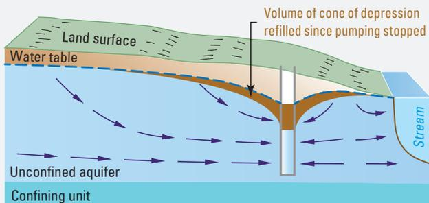
**D.** After pumping stops, groundwater levels begin to recover, and water flows into aquifer storage to refill the cone of depression created by the previous pumping stress.
