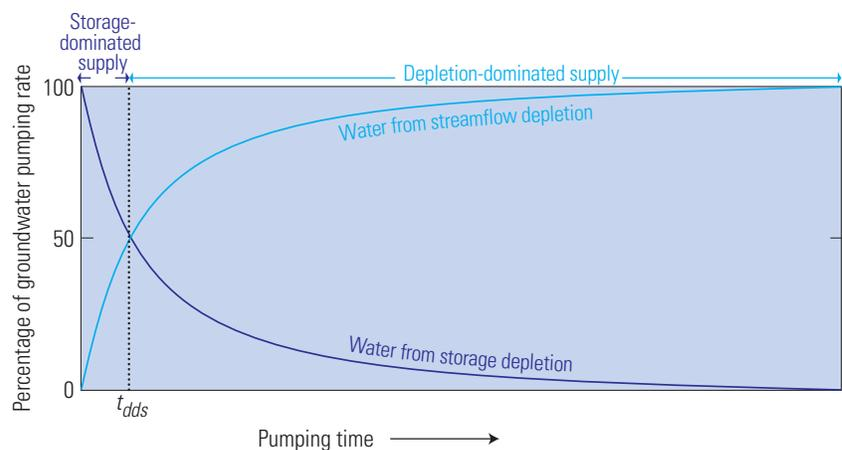
**Figure 2.** Relation of storage change and streamflow depletion as sources of pumped groundwater through time for a hypothetical well. The variable  $t_{dds}$  is the time to reach the condition of depletion-dominated supply for a particular pumping location. In some settings, the transition from storage-dominated to depletion-dominated supply can occur in a matter of days to months, whereas for others depletion-dominated supply may not occur for decades.
