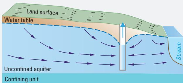
**B.** Pumping from a well removes water from storage in a cone of depression and reduces discharge to the stream.
