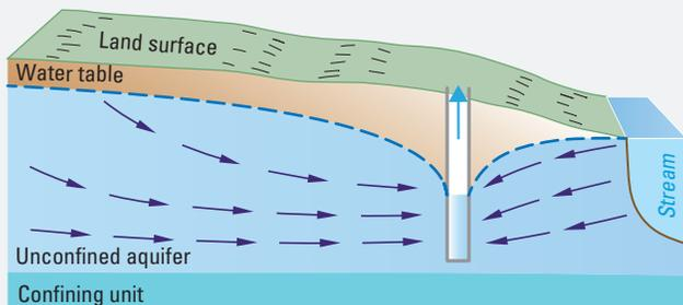
**C.** In some circumstances, the pumping rate of the well may be large enough to cause water to flow from the stream to the aquifer, a process called induced infiltration of streamflow.
