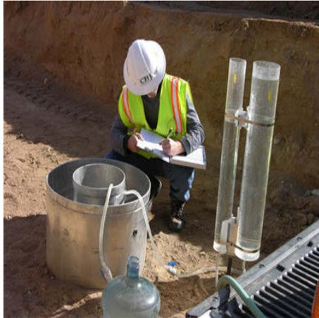
During construction, it is recommended that the infiltration capacity of the subgrade is verified prior to the placement of the stone reservoir. This will ensure that the hydrological condition of the pavement is adequate.
