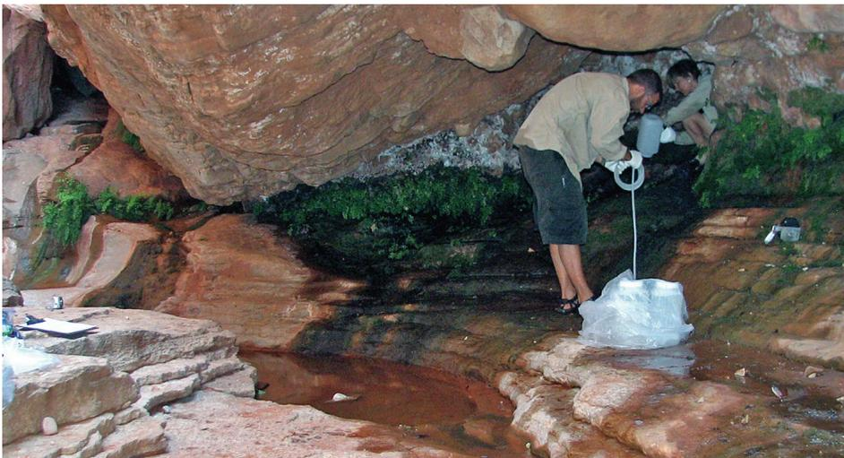
**Figure 4.** USGS scientists taking a water sample at Buck Farm Spring, which was 1 of 20 springs sampled as part of new research to investigate possible impacts of uranium mining in northern Arizona. Sites selected for sampling were designed to fill gaps in historical water-chemistry data in the region. (USGS photo by Nancy Hornewer.)
