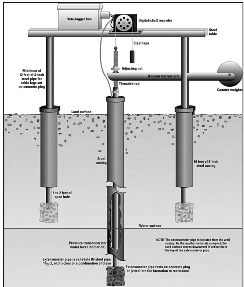
Figure 3. Diagrammatic sketch of a vertical extensometer installation in the Tucson Active Management Area, south-central Arizona.
