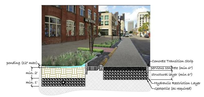
Figure 7. Example downtown streetscape standard for bioretention and pervious concrete
