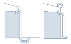
Figure 6 Examples of tank overflow outlets
