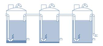
Figure 2 Multiple tanks connected in series
